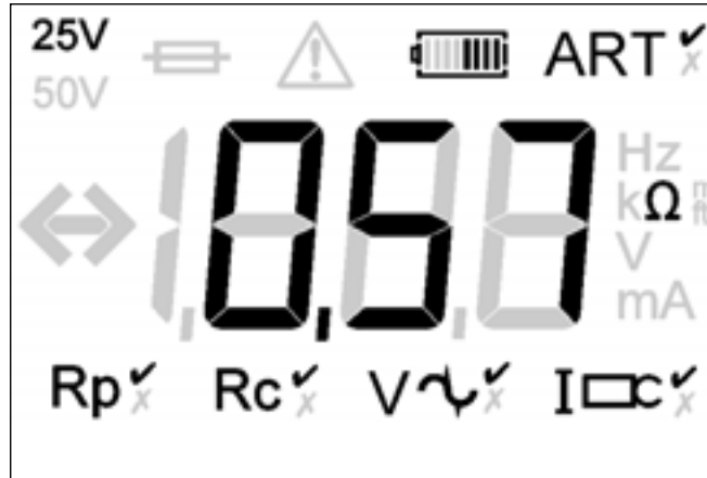
Figure 34: example three-terminal resistance reading with lead-null using ART (DET4 display shown)
