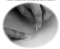
Bio-Tape™ consists of a flexible plastic microscope slide with a pre-defined adhesive area. A center-line marker on the slide aids the user in locating the center of the adhesive when taking the sample and also aids the laboratory analyst in finding the center of the sample area. Each slide is provided with a unique serial number for traceability and packed in a slide mailer to prevent cross contamination.
