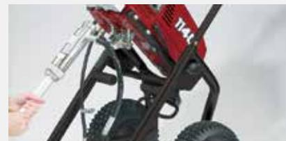
3. Pull handle under body. Slide out fluid section.
