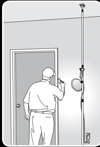
Flood light support
