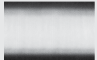
Latex paint through a HEA 517 tip at 1,000 PSI
