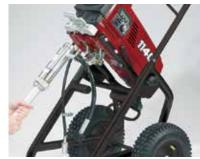
EasyOut<sup>™</sup> Fluid Section T-slot piston and release mechanism makes removal fast and easy. Available on the Impact 1140 only.
