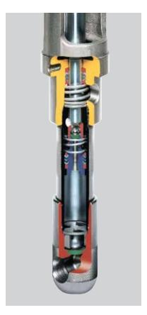
Severe Service<sup>™</sup> 900 Pump Cylinder and piston rod are tempered with a proprietary heat-treating process that increases pump life 150% over competitive pumps. Self-adjusting packings resist over-tightening and help prevent premature wear.
