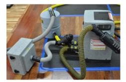
STEP 1: (Left) Install the Interceptor Air In and Out hoses onto the HP unit (as instructed in the Interceptor manual). Remove the Main W from the end of the Air In hose and thread the male end of the Water Separator's hose into the female fitting on the end of the Air In hose.
