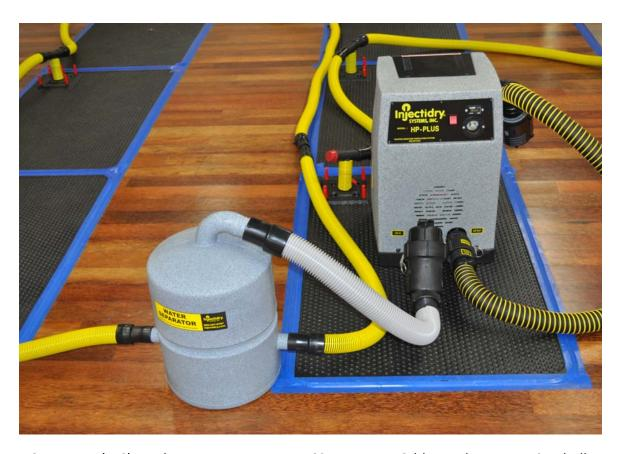
The Water Separator (WS) works to protect your HP60 or HP-PLUS blower by preventing bulk water from passing through it when drying in a negative mode. The WS will collect hidden bulk water that may be trapped in ceilings, walls, floors, or cabinets that you are drying. The WS should be used during the initial phase of your drying job, after water is extracted with a truck mount unit, and should be monitored by a technician.
