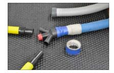
If you do not have a HB300, use tape to temporarily seal the Main W to the end of the extraction line.
