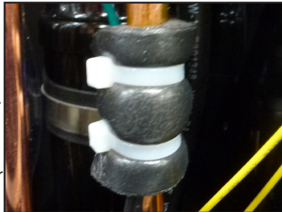
Figure 6: Thermistor attached to the refrigerant line.
