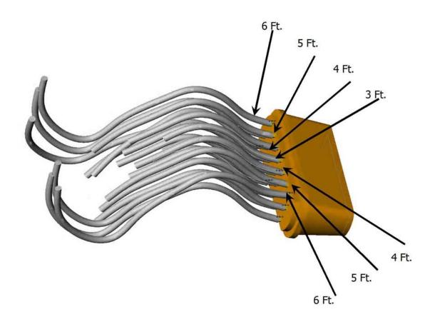
In order to achieve the best air pressure for wall drying, Viking Equipment recommends that the 1/2 X 3/8 inch Vinyl hoses be cut as shown above. Lengthening hoses will result in a loss of pressure unless pressure is equalized by capping-off one or more hoses to compensate. Hose caps are incorporated into the front of the PDS-21, below the Viking logo.
