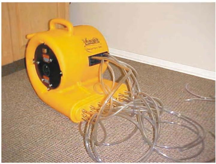
**NOTE\*** END HOSE THAT IS NOT PLUGGED INTO A WALL HOLE MAY BE PLUGGED BACK INTO THE PLUG OFF SYSTEM ON THE UNIT INCREASING THE AIR FLO TO OTHER HOSES.
