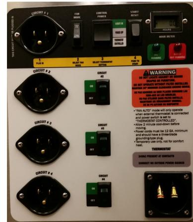
**Start/Reset Switch:** The START/RESET Switch is used to enable the Compact 20 to produce heat. If at any time power to the control circuit is lost or if a fault condition occurs, the Compact 20 will go into the FAULT/NOT RUNNING mode. Pushing the START/RESET switch will energize the control circuit and restart the Compact 20.
