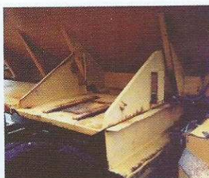
Salt Spreader after 2 years service. Refinished in 2-part Zinc rich Primer and Polyurethane Topcoat.
