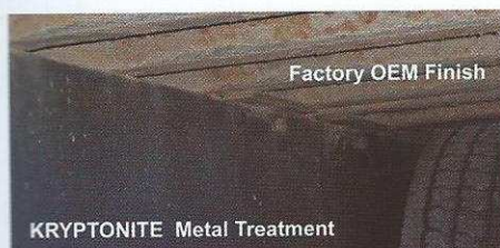
Picture taken of highway transport trailer after 500,000 miles of continuous use from the East Coast to Toronto.
