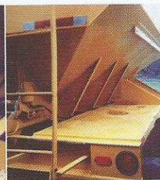
Salt Spreader after 5 years service. Refinished with KRYPTONITE and Topcoated Polyurethane Paint.
