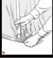
Plastic sheeting can be slippery too, and when it is placed between the pole and the GripDisk<sup>™</sup> it stays locked in place.
