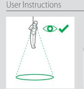
Check the ground below to ensure descent path is clear and a safe landing is possible.
