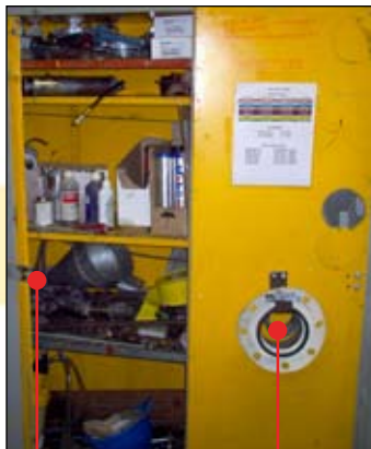
Violation: Padlock hasps or brackets screwed to cabinet
