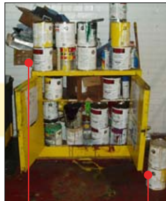
Violation: Flammable items stored outside a cabinet
